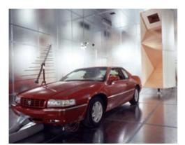
ETS-Lindgren's SMART (Statistical Mode Averaging Reverberation Test-Site) Chambers use the latest developments in proven reverberation technology and experienced chamber design and construction, to create a suitable electromagnetic
